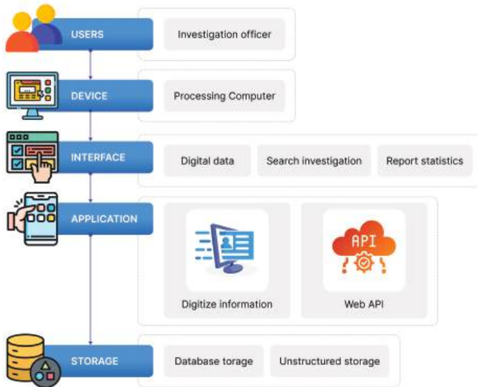
System Model of the Criminal Investigation and Tracing Software
